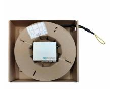
PlasticApartment Optical Termination Box, pre-connected on both sides, with 4 SC/APC sockets and shooter; available with 10m of 4-fibre cable for FTTH multiservice installations; very useful solution to bring inside each individual housing unit all centralized services in the CSOE of FTTH installations. It meets the requirements of class Cca according to CPR EN 50575.
